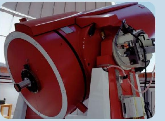
The spectrographs CORALIE and SOPHIE are both state of the art instruments on telescopes in the 1-2 m class with recently installed stabilised FP calibration units put together at the Observatory of Geneva. The FP etalons is placed in vacuum and temperature controlled to achieve highest intrinsic stability of the produced spectrum.
