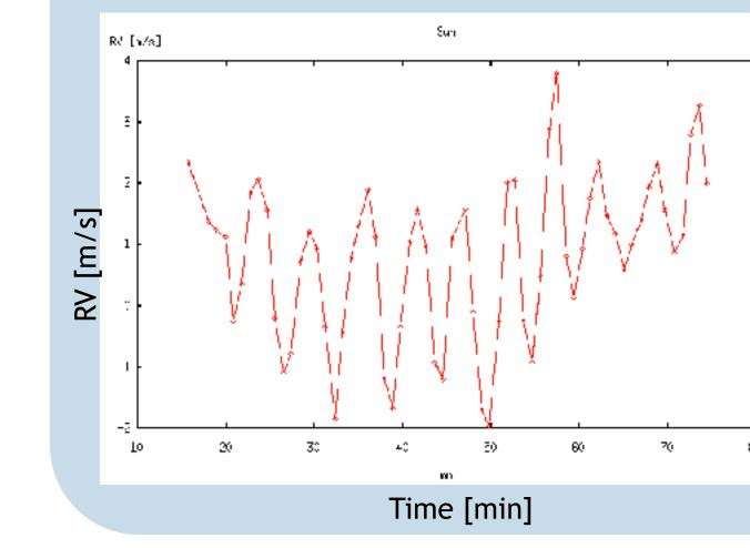
An RV signal of ~5 m/s due to the 5 minute pmode oscillations of the sun, have been measured in a short 40 min sequence on blue sky with 30 sec exposures. This kind of precision has been enabled by the Fabry-Pérot calibration unit.
